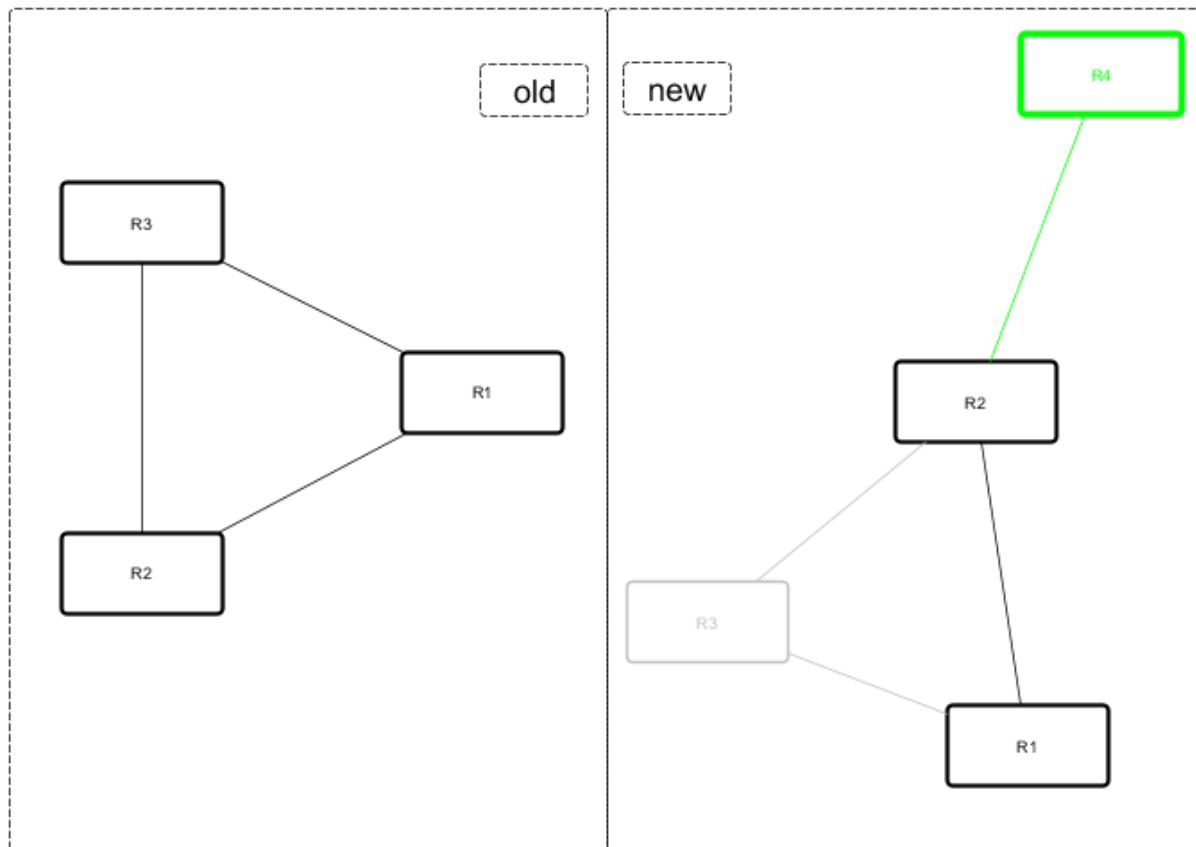
R3 and its links are missing - highlighted in gray, but R4 and its link is new - highlighted in green.
